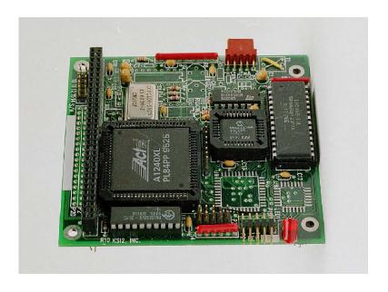
The PC104-SG from Brandywine Communications provides precision time with zero latency to the host computer over the PC/104 bus. An on-board microprocessor automatically synchronizes the clock on the PC104-SG to reference signal inputs. The clock can free run and be preset by commands from the host over the PC/104 bus.
