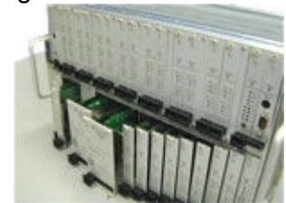
In addition to DS1 and Composite Clock (CC) output cards, any of the 10 main output slots can be equipped with time distribution modules (NTP or IRIG-B) or with DS1 retiming cards. With it's complete and consistent family (6U: 200 outputs, 3U: 60 outputs, expansions, ...), the 5548C is the TSG of choice when you need scalability and reduced spare parts inventory. This flexibility makes the 5548C the most versatile TSG in the marketplace.
