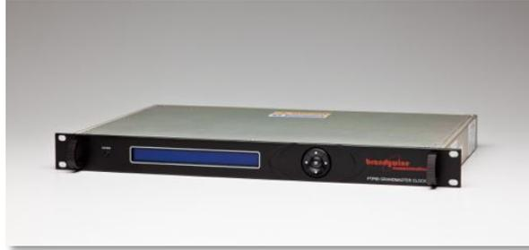
The PTP80 Elite-S GrandMaster & Boundary Clock generates and distributes precisely synchronized time across packet networks. It uses Precision Time Protocol (PTP) to IEEE- 1588 v2 to distribute time to remote PTP clients and slaves over a network. Multiple PTP80 Elite-S units can be utilized for load sharing resilience and increased support. It is also capable of synchronizing to PTP offering further timing resilience.
