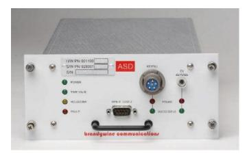
The PTS-SAASM is a state of the art frequency instrument offering a wide range of features and time and frequency outputs accurate to < 40ns  $_{rms}$  to UTC (USNO) and  $1x10^{-12}$  respectively.
