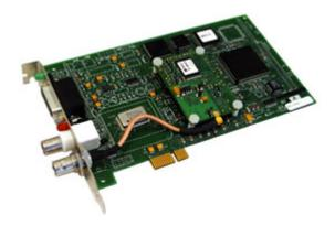
Internal or external processes may be automatically initiated or terminated by using the Match Time feature. This feature asserts an output when the clock's time matches that of the user input start time. The output is terminated under user control or when the pre-programmed stop time is encountered. The resolution of the Match Time comparison is one microsecond.
