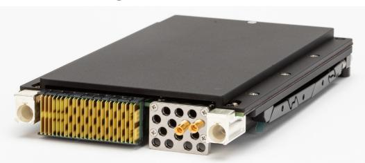
The VPX Timing Card offers a complete solution set for all PNT needs. This ruggedised conduction-cooled unit provides versatile, multifunction, highly-stable clock references for any environment.
