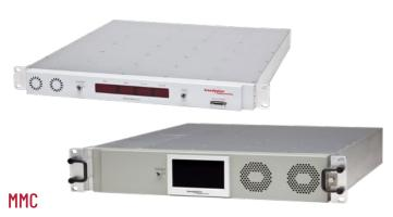
Brandywine's Modular Master Clock (MMC) represents the next generation of modular timing systems. MMC provides assured timing capabilities using Brandywine's Timewall™ technology incorporating multiple clock inputs from GPS/M-code, cesium to two-way satellite time and frequency transfer (TWSTFT).
